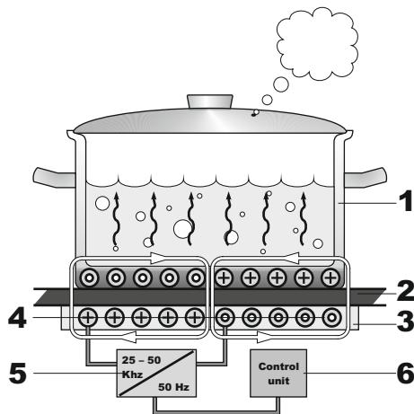
1. Utensil made of ferromagnetic material
